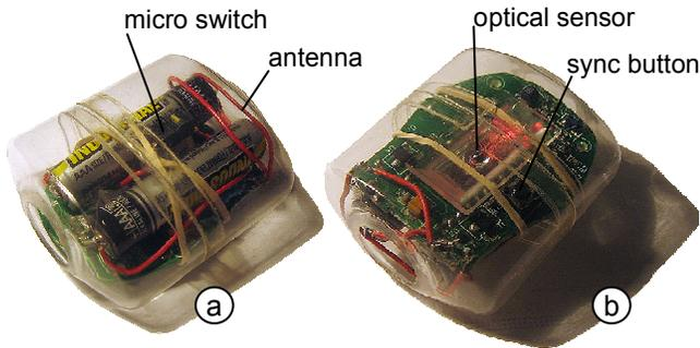
**Figure 3** The soap core (a) top & (b) bottom view. A micro switch in a slightly elastic casing allows users to generate a click by squeezing the device.
