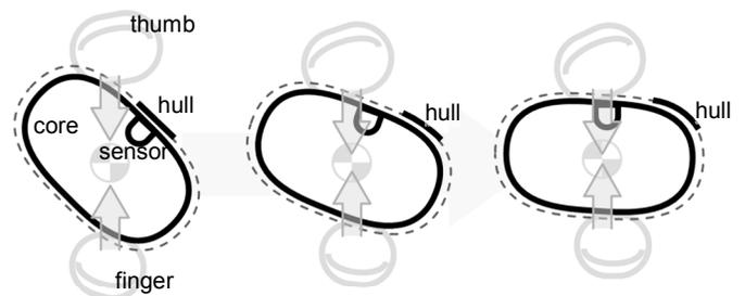
**Figure 2** The mechanics of soap: As the user applies pressure using thumb and finger, the core rotates to evade the pressure. At the same time, friction between finger and hull holds the hull in place, resulting in relative motion between hull and core.
