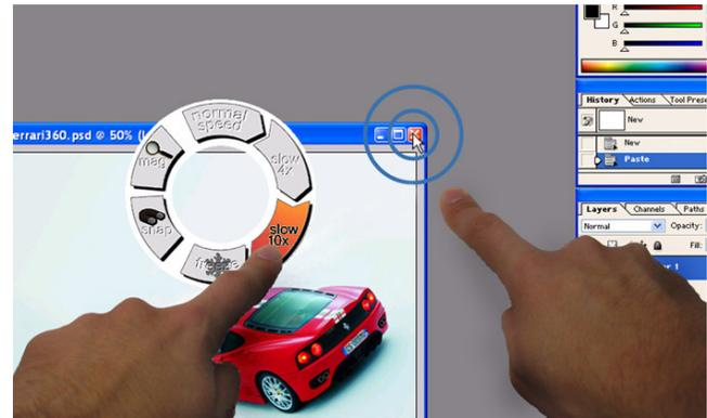
**Figure 1. Precise dual finger selection techniques enable pixel-precise selections and manipulations on multi-touch screens. This image shows the use of Dual Finger X-Menu in selecting “slow 10X” mode.**
