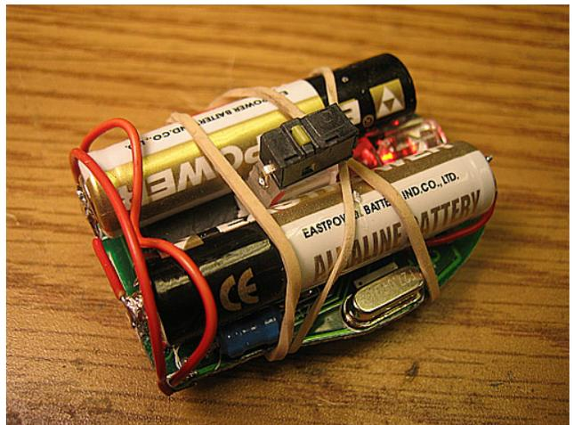
**4. Assembly:** Cut a hole into the filling material to make space for the micro switch. Then put the filling material on top of the device and slide it into the casing. Double check that pressing the casing triggers the micro switch.
