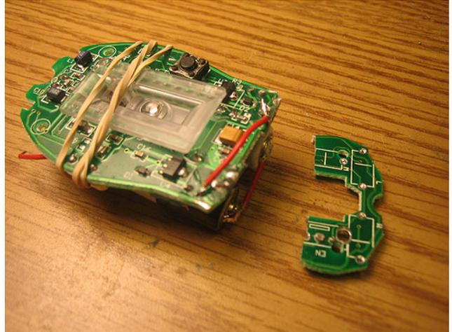
Scrape of some isolation and solder the mouse button connection straight onto the board. Do the same with the conductive paths serving as the antenna (top and bottom of the board).
