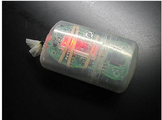
Stick the core with its first hull into the second hull and fill the lubricant between the two layers. To avoid bubbles, use plenty of lubricant at first to push out the air, then push out surplus lubricant before sealing the second hull. The amount of lubrication is an optimization problem. More lubricant means that your soap will be easier to operate, but also moves the hull further away from the optical sensor and might lead to tracking errors.
