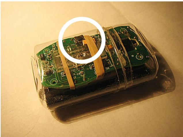
Use the clear adhesive tape to seal the casing.
