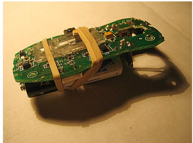
Without the mouse casing the batteries will sit lower. Use the pliers to adjust the battery connectors to fit the new height.
