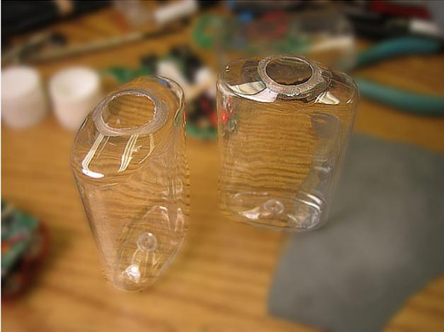
For the gaming soap we used the bottoms of the two casings. Cut them to roughly the right length; use different lengths to make sure the seam won't be over the sensor.
