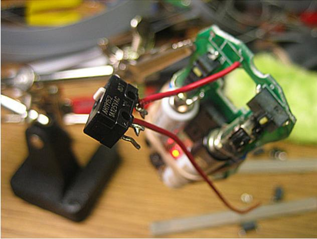
You will now move it to the center of the device. Adjust the height of the block of plastic/wood, you will use it to prop up the micro switch such that it reaches the inside wall of the casing. Mount the block on the back of the chip between the batteries using the two-sided tape; then mount the micro switch on top of it. If you are making a gaming soap, connect the micro switch with its original location on the board using two cables of matching length.
