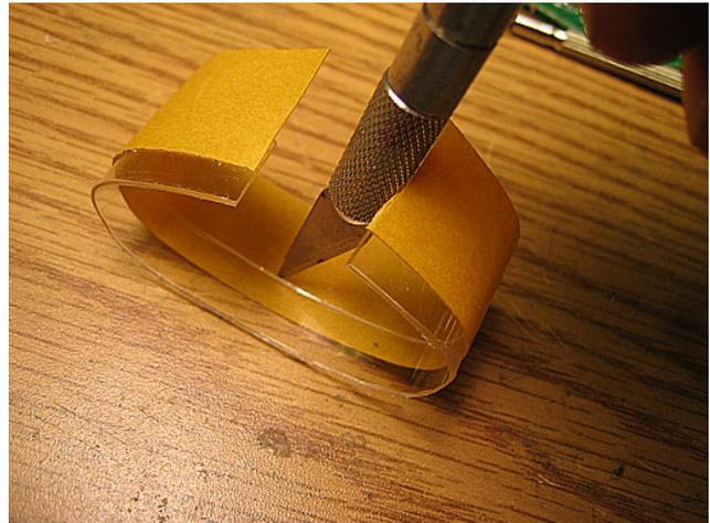
Glue the remaining open ring half-way into the shorter part of the casing using double sided adhesive tape. This will strengthen the casing and make sure the two halves stay aligned.
