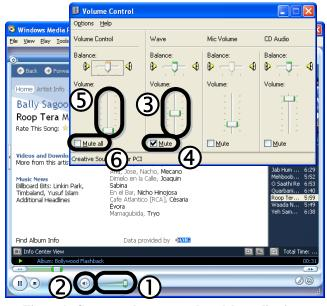
Figure 1: Current volume control model: application audio output is only active when its volume slider (1) and wave and master sliders in the control panel (3, 5) are set to non-zero values and the three mute check boxes (2, 4, 6) are unchecked.
