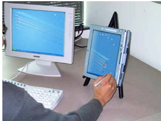
Figure 4: Drag-and-pick allows users to temporarily move icons from an external monitor to the tablet where the user can interact with them using the pen.
