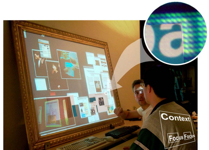
Figure 1: ContextWall prototype. The iconic illustration (bottom right) shows the location of the two embedded focus screens. The callout shows the different resolutions of focus and context areas.
