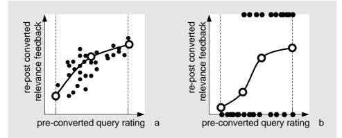
Figure 16: Enhanced weighting function. A spline with free knots approximates (query ratings, relevance feedback) tuples. Example with three free knots and real-valued relevance feedback (a) and with four knots and Boolean feedback (b).
