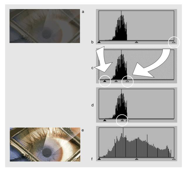
Figure 26: Adjusting luminance distributions using a histogram-based dialog.
