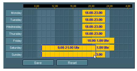
Figure 49: A paintable timer interface. It allows users to input intervals for a whole week.
