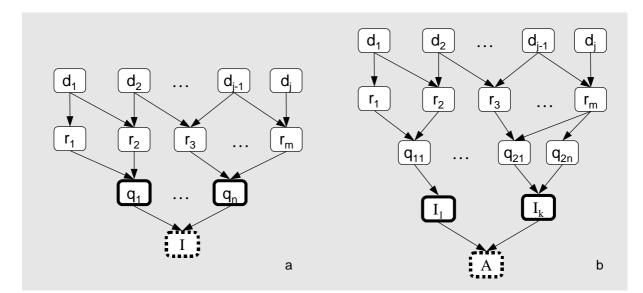
Figure 13: Inference networks (four-layer version, [TC92, p. 282]) may be used to support a QuerySet Architecture (a). QSA-enhanced inference network (b). Thick-bordered nodes implement QSA queries, dashed nodes the aggregation function. (d = document nodes, r = concept representation nodes, q = query representation nodes, I = Interest node. A = Aggregation node)
