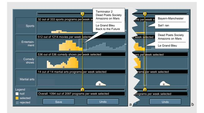
Figure 36: A histogram-based profile editor applied to the TV domain. This prototype of the TV Scout profile editor illustrates histograms with lists of example objects.
