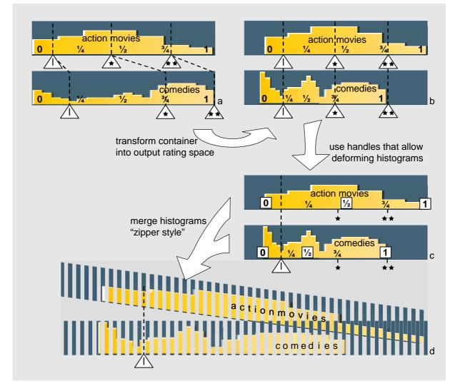
Figure 30: Transforming histograms (a) into output rating space (b) and application of histogram-attached handles (c). Since horizontal positions now represent the same output rating scale, the two weighted histograms can be merged visually (d).
