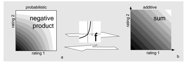
Figure 15: Conversion between probabilistic (a) and additive rating scales (b).
