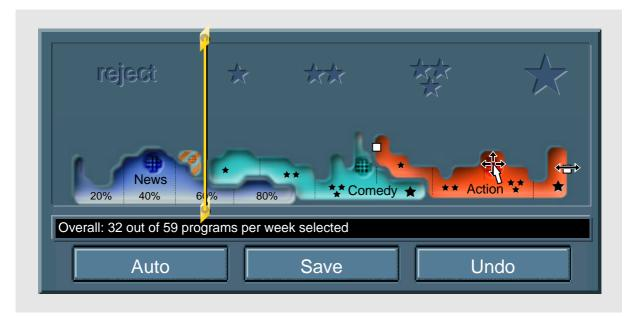
Figure 37: Profile editor using a histogram stack, jelly look. Jelly histograms can be manipulated by dragging them horizontally (shown as a cross cursor) or by grabbing one of the handles attached to a histogram's edges (white squares) and dragging them, which moves only this edge so that the histogram is deformed (shown as a double arrow cursor).
