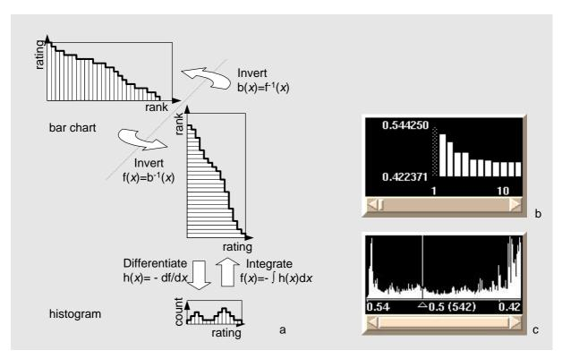
Figure 33: Histograms provide the same information contained in bar charts, and can be converted into each other (a). Histograms are more compact. While bar charts represent each object as a bar, histograms use only a single "grain" to represent each object. By varying the number of bars, histograms can be miniaturized to any size. While a bar chart (Xinquery [CCH92, INQUERY92]) can only show the ratings of a subset of a large ranking (b), a histogram can give an overview over *all* objects (c).
