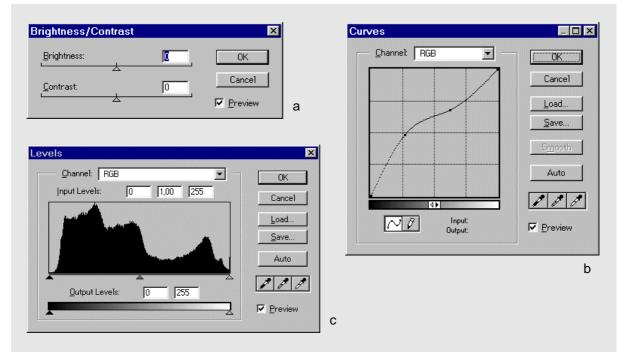
Figure 23: Brightness/contrast dialog (a), graduation curves dialog (b), and levels dialog
