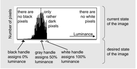
Figure 25: The histogram component that is part of the levels dialog visualizes the current luminance distribution of the image (top half) and allows assigning new luminance values to groups of pixels (bottom).
