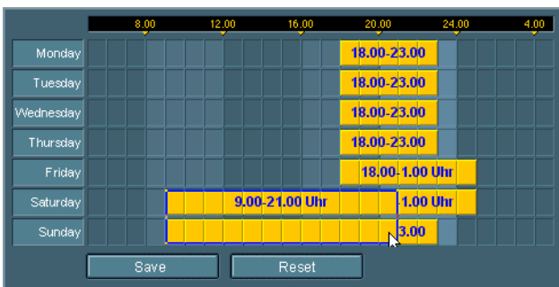
Figure 7: A toggle map timer interface. It allows users to input intervals for a whole week.
